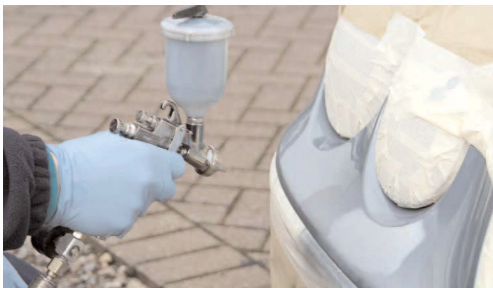
Figure 2 Typical SMART repair
